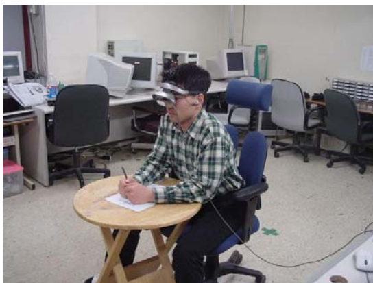
Figure 4: A Group II subject viewing the virtual environment with a head-mount display (the black drape cover is not shown for illustration purpose).
