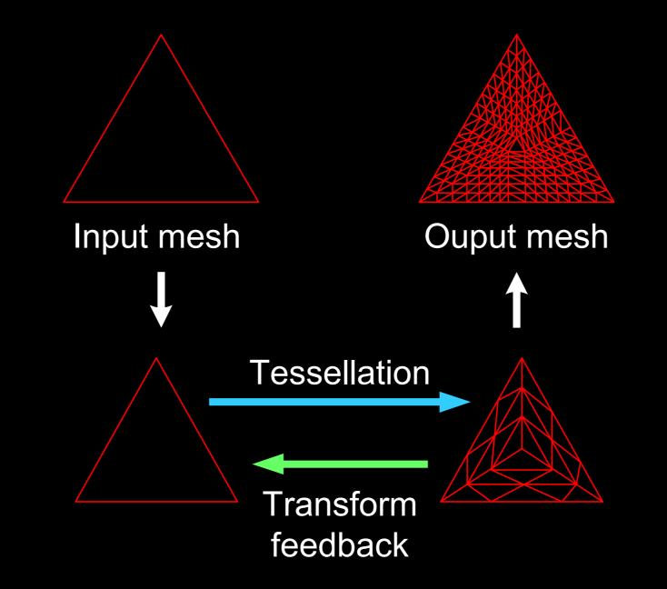
**Recursive Tessellation** Multi-stage tessellation, combining tessellation and transform feedback (or stream-out in Direct3D), allows us to (virtually) infinitesimally subdivide a coarse mesh beyond typical hardware limits, which can lead to extremely detailed geometric representations.
