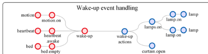
Fig. 5. The hierarchical view visually summarizes sensors, actuators, and their mapping.
