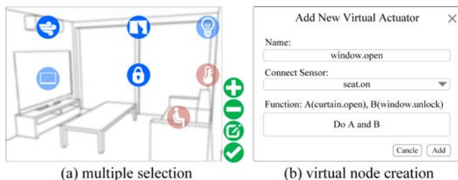
Fig. 4. Multiple nodes (here, strong-blue actuators) selected by a user (a) can be grouped to form a new virtual node with its behavior definition.
