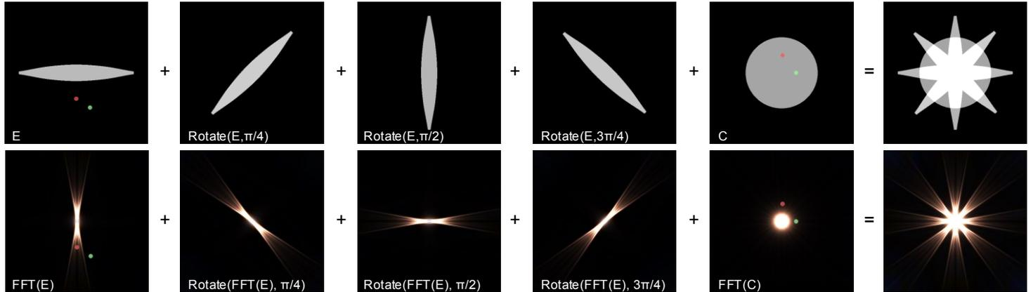
This poster presents a novel scheme of diffraction synthesis, which additively integrates diffraction elements with fast Fourier transform. We decompose a aperture shape into atomic geometric elements to abstract diffraction features. Curved blades (E) and circular core (C) abstract non-symmetric streaks and core highlights, respectively.
